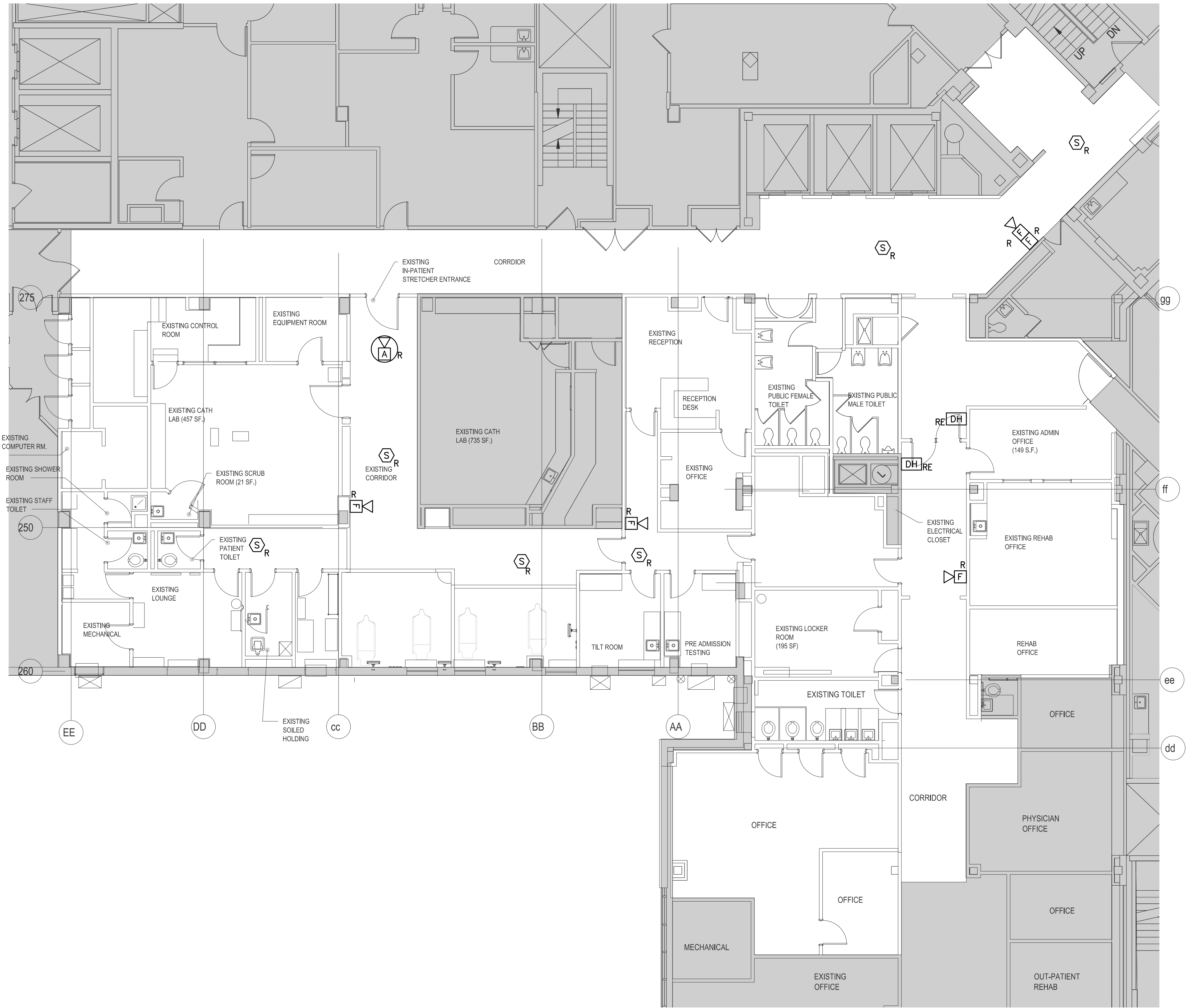
1 FIRE ALARM DEMOLITION 1ST FLOOR PART PLAN SCALE: 1/8" = 1'-0"
